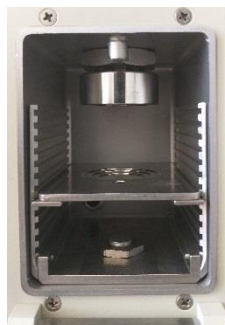
A Chamber of alpha spectrometer, detector and sample holder
